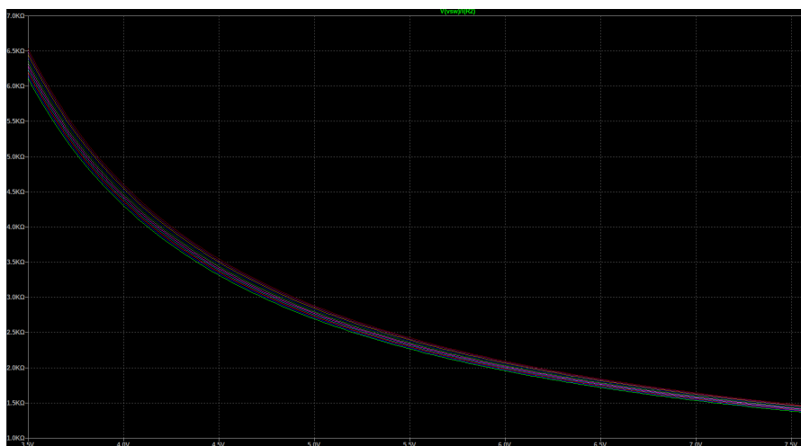
Figure 1: M2 biasing and variable resistance with gate-to-ground voltage
